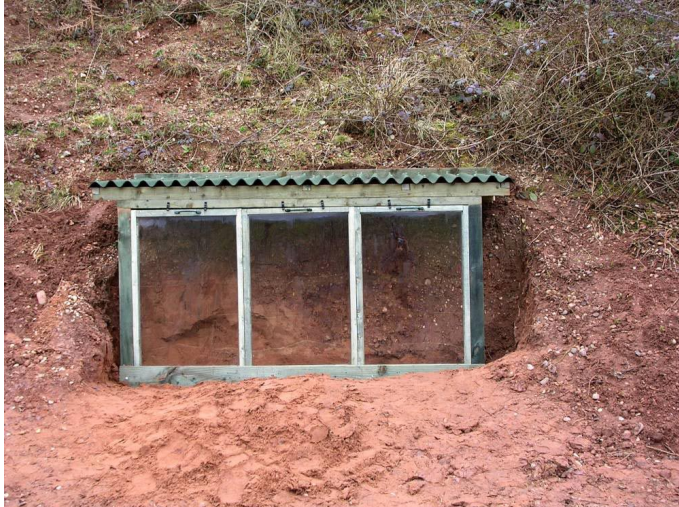
Fig: 2 Experimental cover to protect Sand / Till contact
